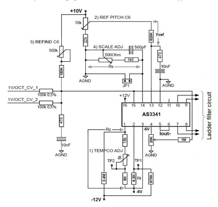
Steps of trimming of AS3341 in ladder filter could be as follow:
